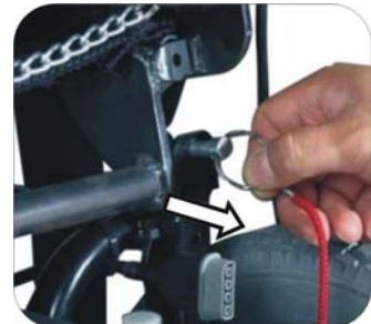
6. Pull the pins out from both sides of the mounting bases.
