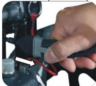
5. Remove the cable from the transmission connector.
