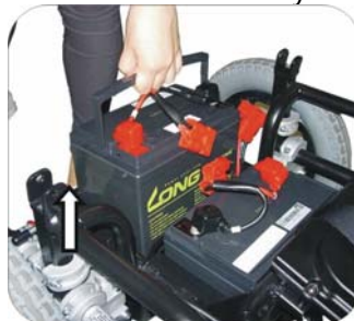
11. Lift up the battery by its handle.
